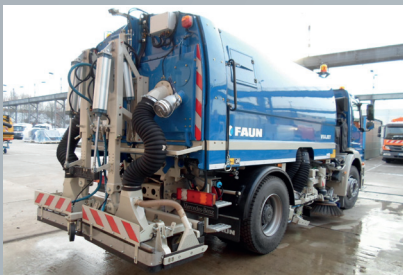
Rear-mounted suction systems (underbody or tailgate mounted)
