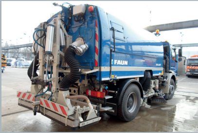
Rear-mounted suction systems (underbody or tailgate mounted)
