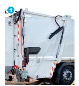
The internally located cylinder and the closed guide rail, made of highly wear-resistant steel, mean there are no openings in the tailgate which might allow waste to fall out of.
